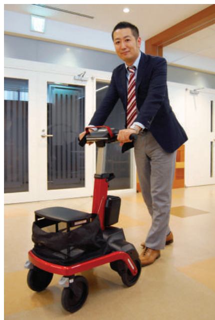
Robot Assist Walker RT. 1, developed by Osaka-based RT. Works Co., is an autonomous walking-assist electric cart.
