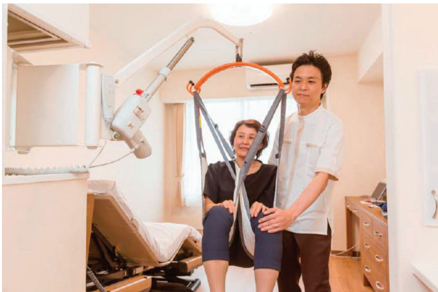
Swing Lift CoCoRo, developed jointly by Orix Living Corp. and Moritoh Co., lifts a woman using an arm capable of making a 360-degree turn. | ORIX LIVING / KYODO
