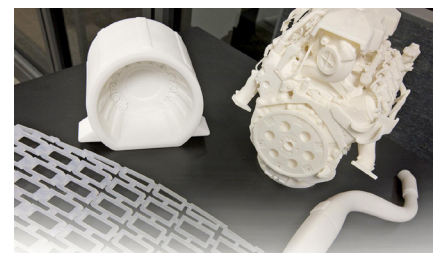
These prototype parts were made with 3D printers at General Motors' tech center in Warren, Michigan.
