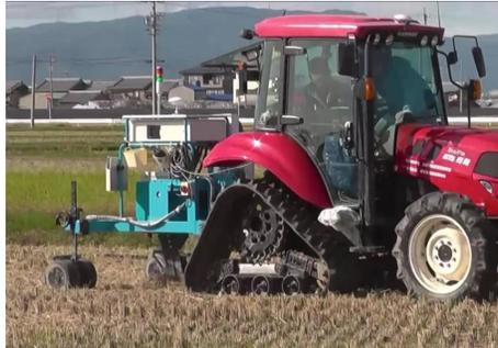
*A tractor tows an optical sensor that can measure the amount of light the soil around it absorbs. | Courtesy Of Toyota Motor Corp. / Via Chunichi Shimbun*
