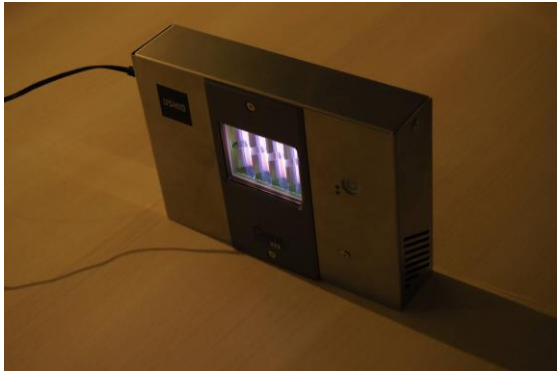
Ushio Inc.'s Care 222 ultraviolet lamp emits specific UV rays whose 222-nanometer wavelength kills the new coronavirus but is safe to humans, as opposed to conventional UV rays which cause cancer and other health problems. / KYODO
